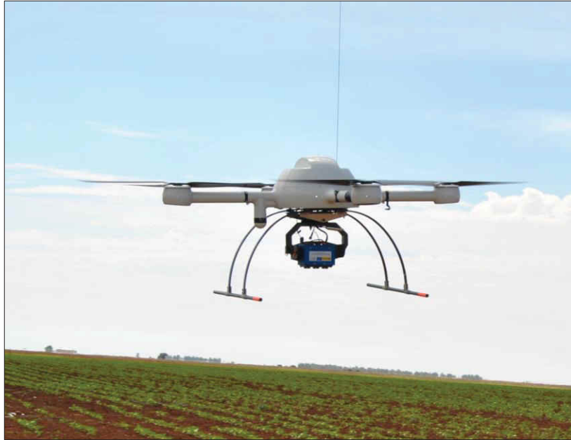
Figure 1. Microdrone MD4-1000 with the multispectral camera (6 channels) embedded flying over one the sunflower experimental fields.
